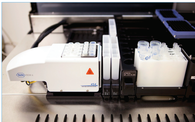
▲ Figure 2: The REM e System can be installed onto commonly used liquid handlers, such as the Hamilton STARlet shown above.
