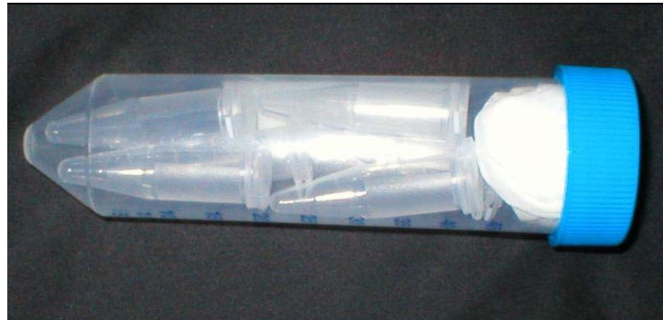
Figure 2. Preparation of microfuge sample tubes for shipping. Place up to six tubes inside of a 50 mL centrifuge tube. Secure the microfuge sample tubes by packing the tube with a paper towel or tissue paper.
